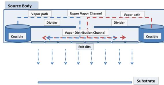
**Figure 1:** Schematic of the VPT Linear Vapor Source
