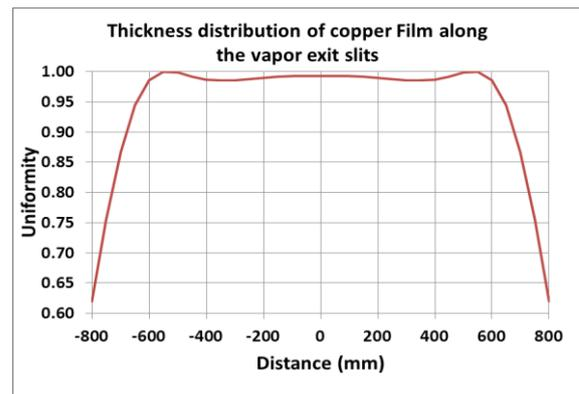
**Figure 3:** Simulated uniformity of the Vapor Source with  $\pm 0.7\%$  thickness uniformity in the 1200mm center region.
