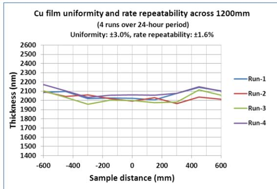
**Figure 5:** Thickness uniformity and repeatability of Cu films
